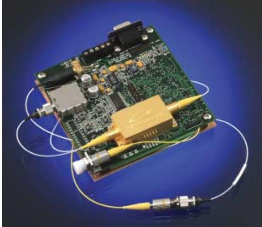
Figure 6. The OSA engine. Dimensions are 110 x 110 x 18.5mm.
